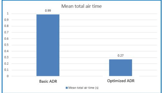
Field tests show significant reduction (-72%) of average total air-time per uplink frame counter.
