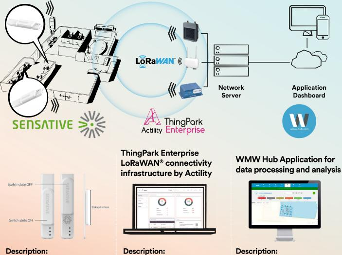
Strips Presence is an innovative ultra-thin (3mm) active IR occupancy sensor for smart offices and buildings. Strips Presence monitors the desk occupancy rate by measuring objects and people within close range (configurable up to 50 cm). It has a unique functionality with a manual interaction stage using +Switch.
