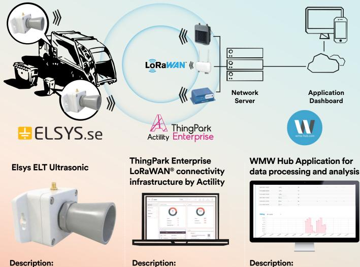
Enclosed in an IP67 box and designed to be mounted outside, ELT Ultrasonic is the ideal wireless sensor for measuring in advanced places or extreme weather conditions and has the capacity of measuring distance with a remarkably long range. Distance report is leveraged by temperature, humidity, and atmospheric pressure data.
