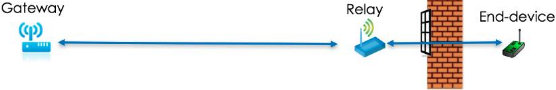
Relaying messages for an end-device behind an extra-thick wall of a building
